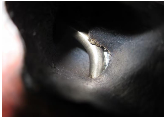
Figure 9: Bent Intake valve stem
