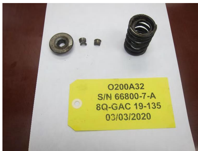
Figure 4: Affected intake valve springs and valve keys
