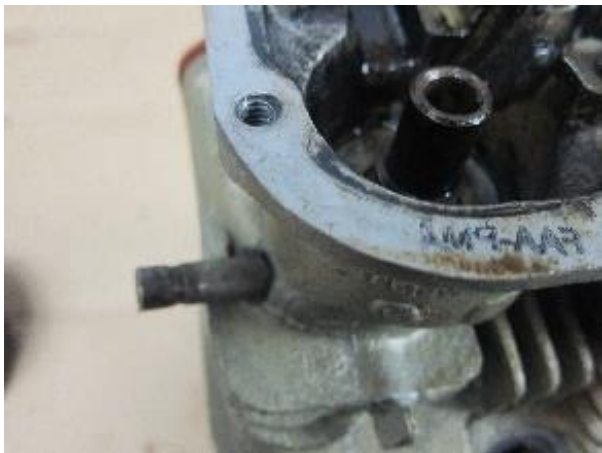
Figure 10: Intake valve stem protruding from the cylinder
