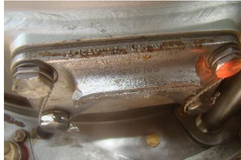
Figure 12: Right Hand engine – One engine vibration isolator (Inboard) was sheared,
