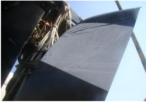
Figure 17: RH propeller blade - red paint scratch marks found possibly due to hitting the engine bottom cowl
