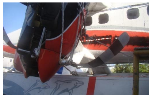
Figure 16: RH propeller blades bent (backward)
