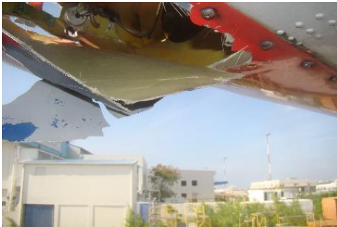
Figure 5: Damage to LH Wing - from rib 25 to rib 28, and wing tip were damaged
