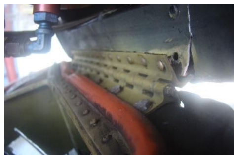
Figure 22: RH cowling – Rivets sheared
