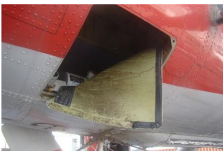
Figure 23: LH Hydraulic bay panel found twisted and bent
