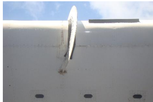
Figure 8: Wing fin dislocated and the leading edges bent inboard
