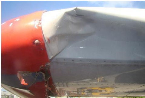
Figure 7: Damage to LH wing - dented
