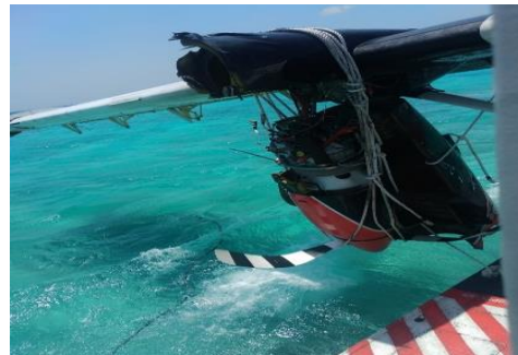
Figure 10: Right Hand engine – completely detached from the mount/nacelle
