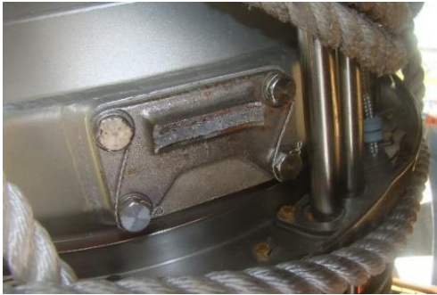
Figure 11: Right Hand engine – One engine vibration isolator (Inboard) was sheared,
