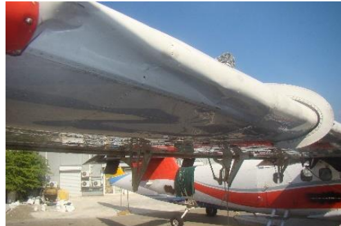
Figure 6: Damage to LH wing - leading edges of rib 26, 27 and 28 buckled
