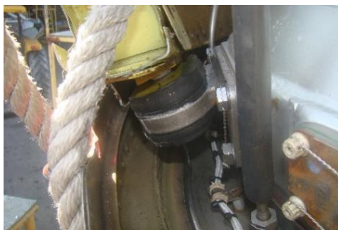
Figure 15: Right Hand engine – both the outboard and top engine vibration isolator (mounts) attaching structures ripped off
