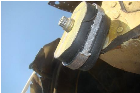
Figure 13: Right Hand engine – One engine vibration isolator (Inboard) was sheared,
