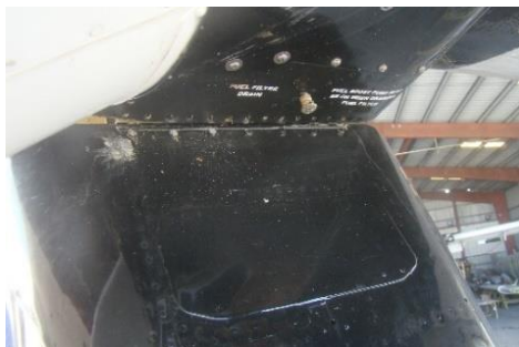
Figure 21: RH engine bottom cowl - attachment rivets were found sheared
