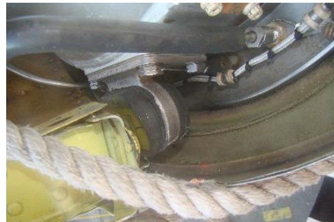
Figure 14: Right Hand engine – both the outboard and top engine vibration isolator (mounts) attaching structures ripped off
