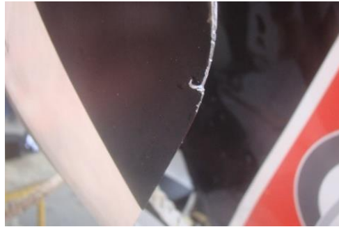
Figure 18: RH propeller – nicks observed on all three blades
