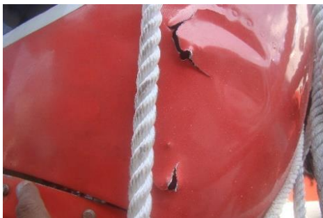
Figure 19: RH engine bottom cowl - skin ruptured at several places
