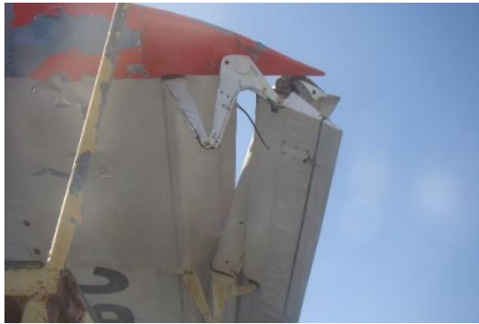
Figure 25: LH aileron (outer most) was twisted and bent upward
