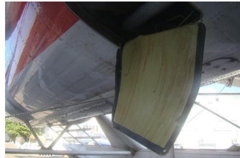
Figure 24: RH hydraulic bay panel found twisted and bent outward
