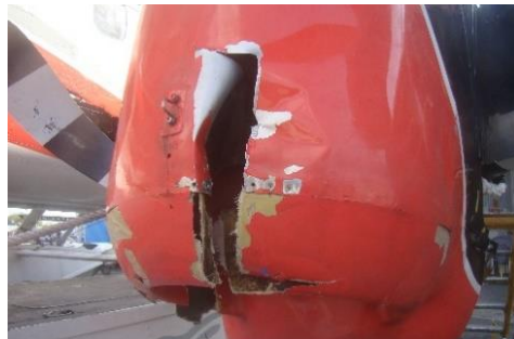
Figure 20: RH engine bottom cowl – prop blade struck through
