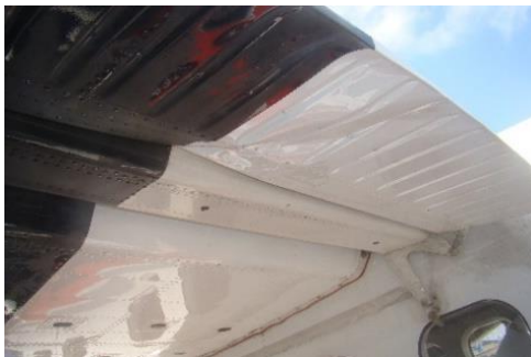
Figure 9: RH Wing - trailing flap skin buckled inward
