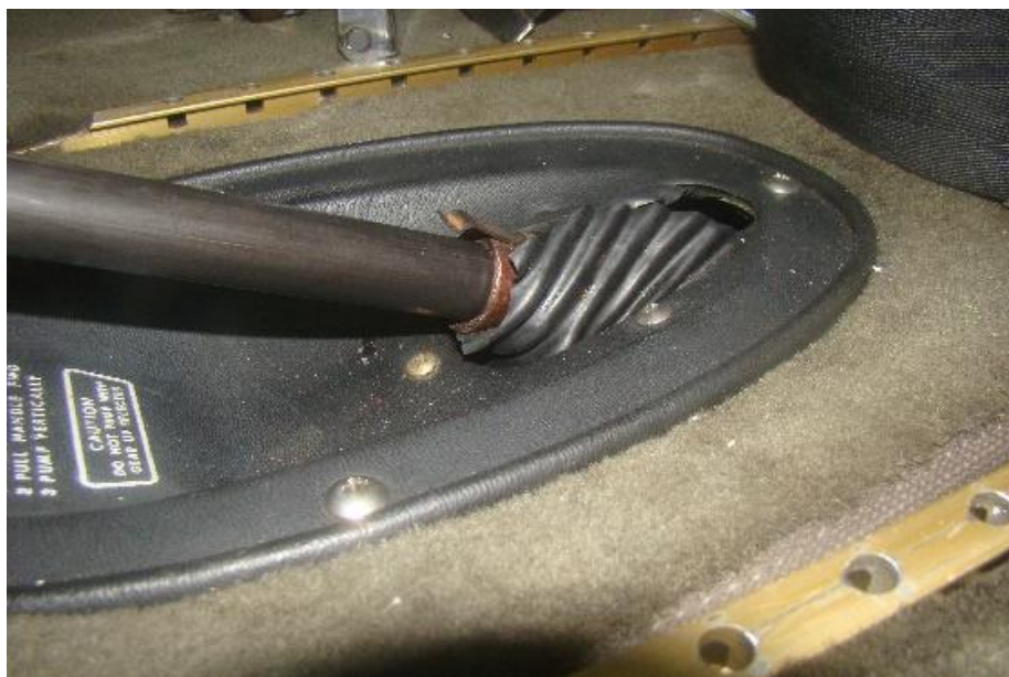
Figure 6: Handle for manual operation of Landing gear
