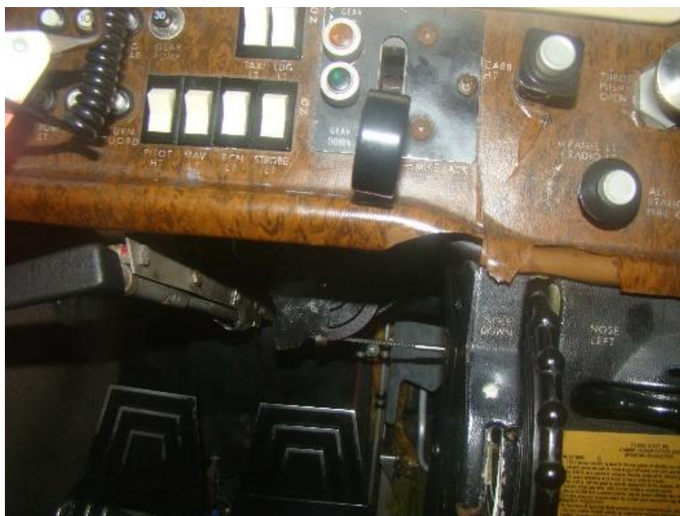
Figure5: landing gear selector switch and gear position indicator lights
