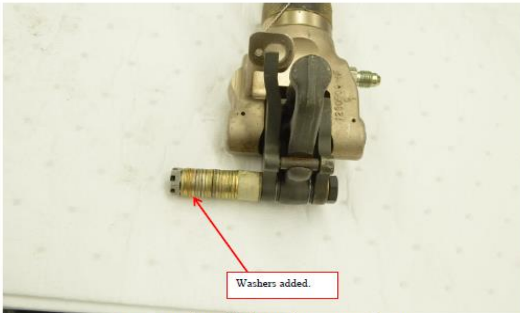
Figure 2 Washers Added to Simulate Gear Attachment
