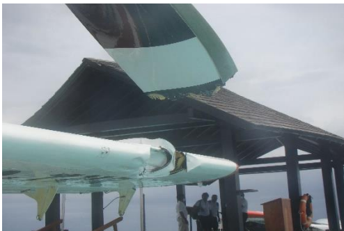
Figure 5: LH Wing: Damage to LH Wing
