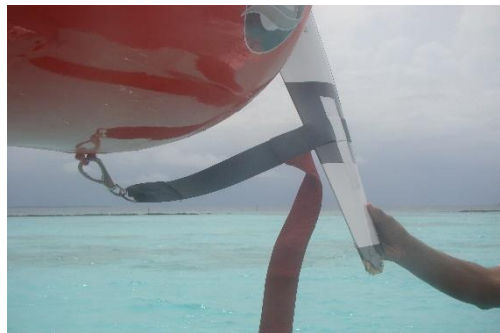
Figure 8: LH Propeller damaged
