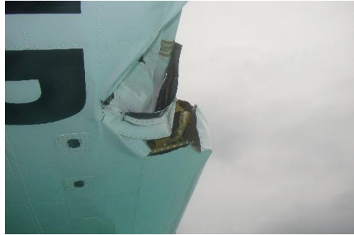
Figure 4: Damage to LH wing
