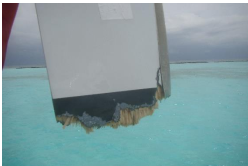
Figure 9: LH Propeller damaged
