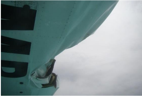
Figure 3: LH Wing: Damage to LH Wing
