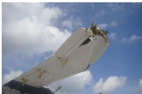
Figure 7: RH Wing: Damage to RH Wing
