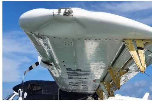
Figure 10: Damaged LH Wing tip
