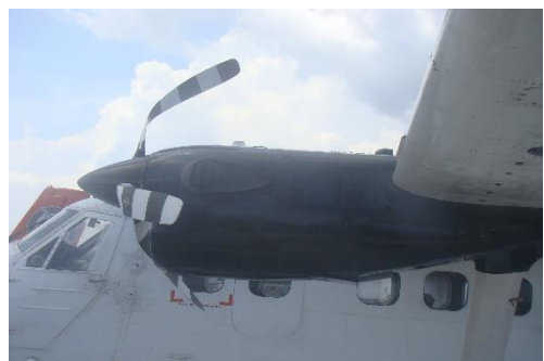
Figure 8: Damaged LH Propeller
