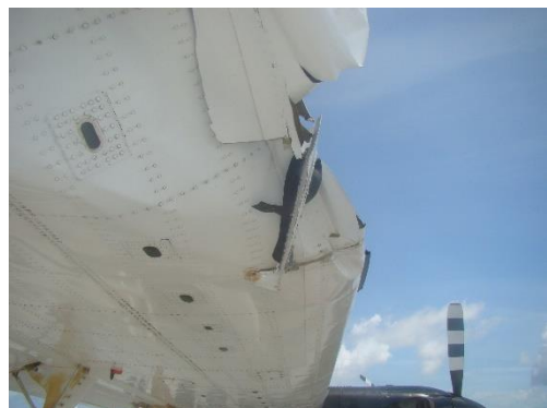
Figure 6: RH Wing: Damage to Wing Leading Edge
