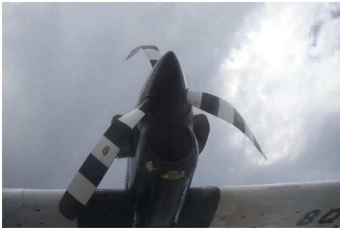
Figure 9: Damaged LH Propeller
