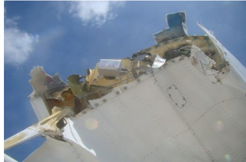
Figure 4: Damage to RH wing tip
