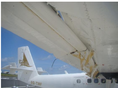
Figure 5: RH Wing: Damage to RH Aileron
