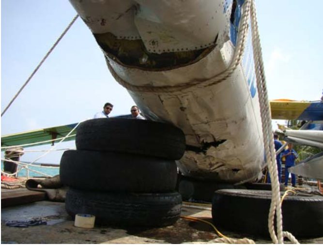
Secondary damage by current, reef and waves
