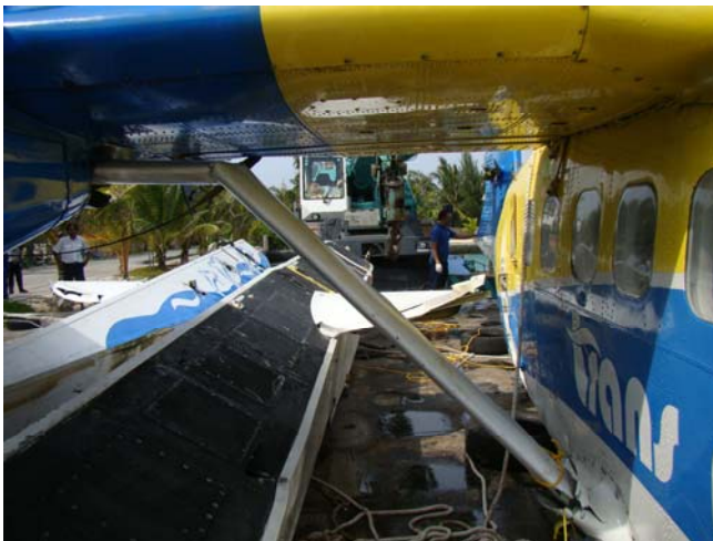
RH wing strut damaged
