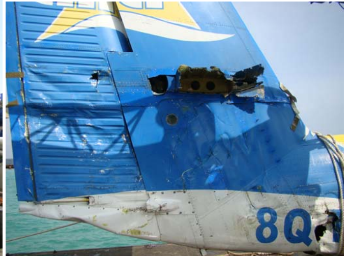
Damage during salvage operation
