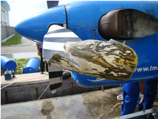
RH Propeller blades bent and some parts worn off
